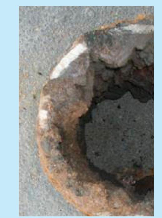
The pipe at left was rejected because of its thin, weak wall.
